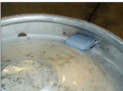
Each keg is fitted with an EPC Gen 2 passive UHF tag made by Confidex.
