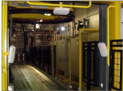
After a pallet of filled kegs is wrapped in plastic film, it passes through the fixed interrogator portal that reads the unique ID number encoded to each keg tag.
